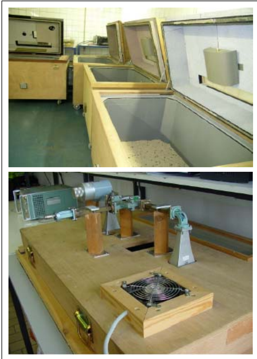
Figure 1 Top photo: overview of the exposure boxes. A 970 MHz antenna may be seen on the inside of the lid of the front box. Bottom photo: Exterior view of the 9.70 GHz box with two horn antennas in the closed lid. Source: thesis Adang. 1
